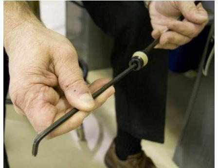
**1.3 Allow fluid to flow out of the coupling until a steady clear stream is observed.** Remove the tool and allow the coupling to close. Check to be sure the reservoir is at least one half full. Check to be sure the "O" Ring on the outside of the coupling is present, clean and undamaged.
