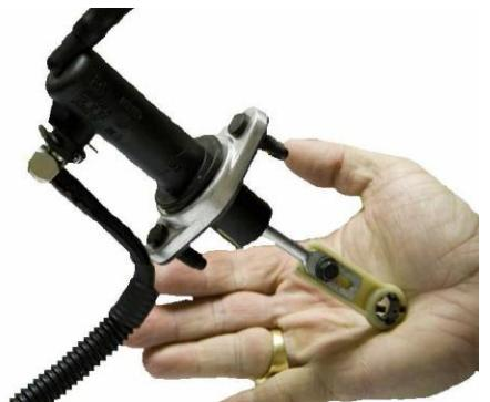
**1.4 Keeping the reservoir end of the M/C pointed up, slowly depress the P-Rod.** Observe the reservoir for signs of air being expelled from the M/C. Repeat this until the P-Rod can only be pushed 2mm before encountering a substantially higher load. If the P-Rod load is still very low, repeat steps (3.2) and (3.3), until only 2mm of free play remain.
