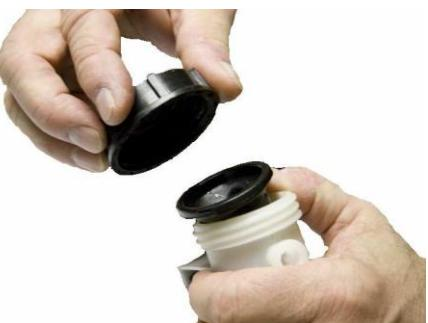
**1.5 Top up the reservoir with brake fluid. Replace the diaphragm and cap onto the reservoir.** Check to be sure the "O" Ring on the outside of the coupling is clean and undamaged.
